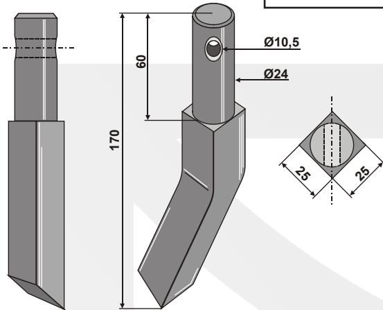
Rotorzinken / dent rotative / rotary tine
